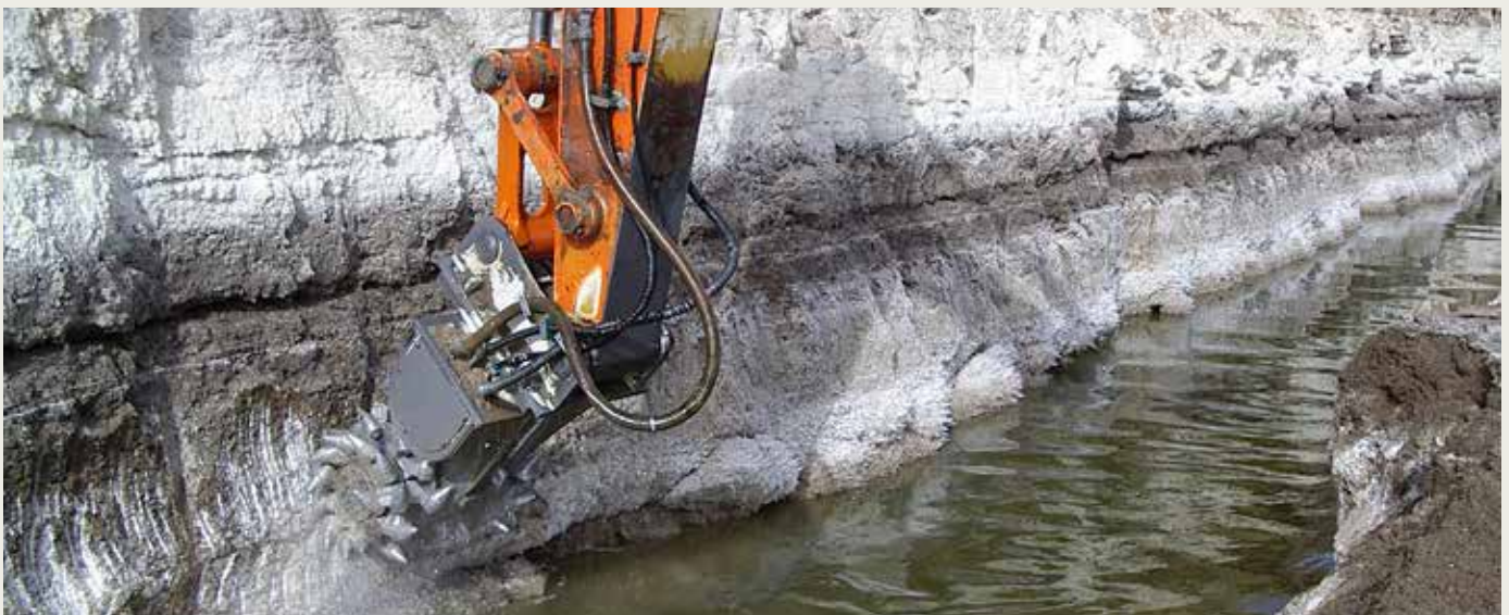
Salt mining with ER 1500-1 in China cutting drainage channels in brine solution
