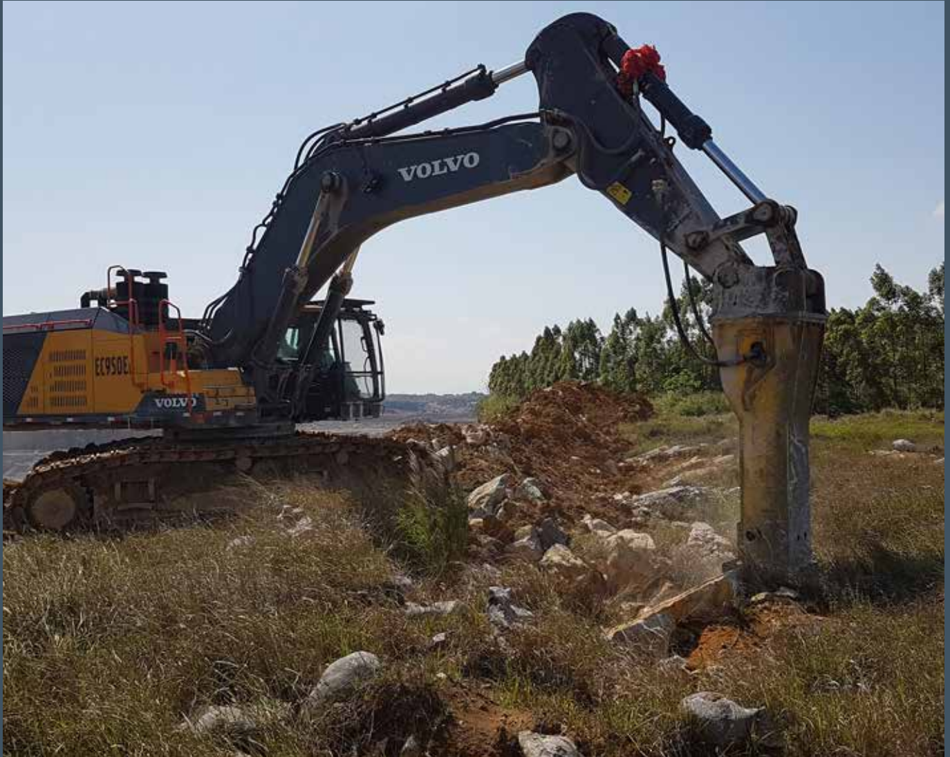
HB 10000 on a 92t excavator breaking limestone boulders in the overburden
