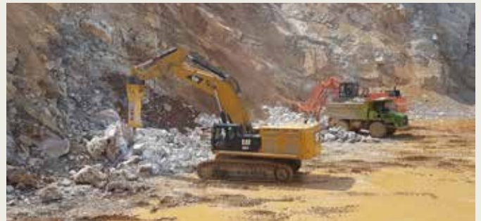
HB 10000 on a 90t excavator reducing boulders in limestone quarry in China
