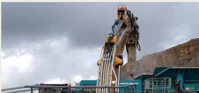
HB 4100 on a 40t excavator helping to remove the blockage in mobile crusher
